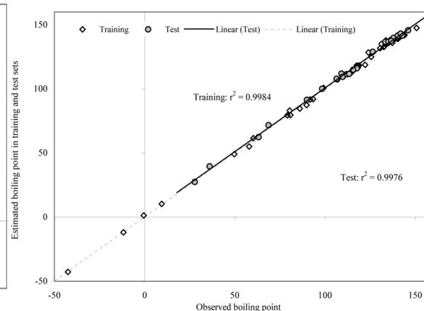
Fig. 2. Training (48) vs test: estimation of boiling points
