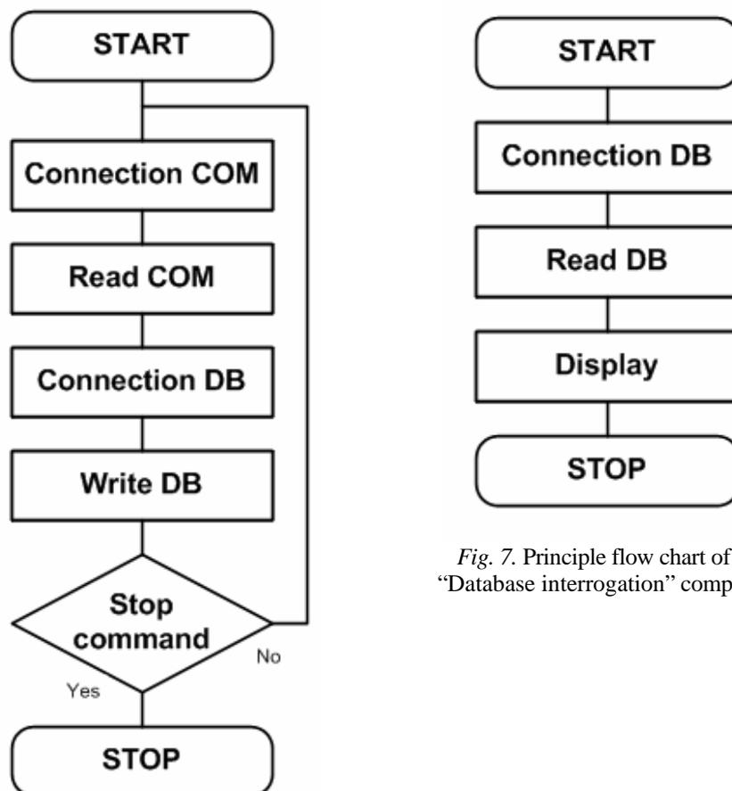
*Fig. 6.* Principle flow chart of the “Acquisition software” component
