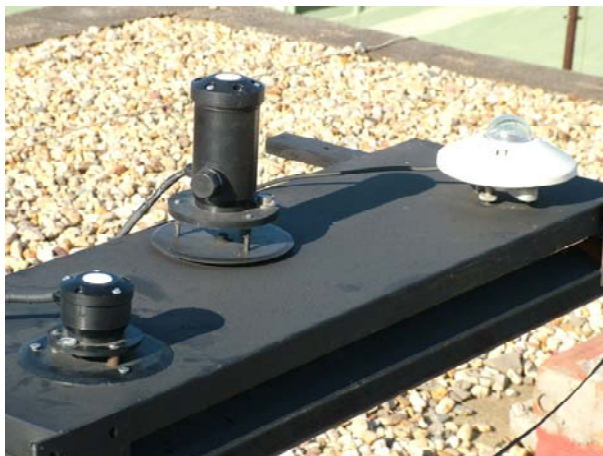
Figure 8. Location for calibrating the two pyranometers constructed, in relation to the standard pyranometer.
