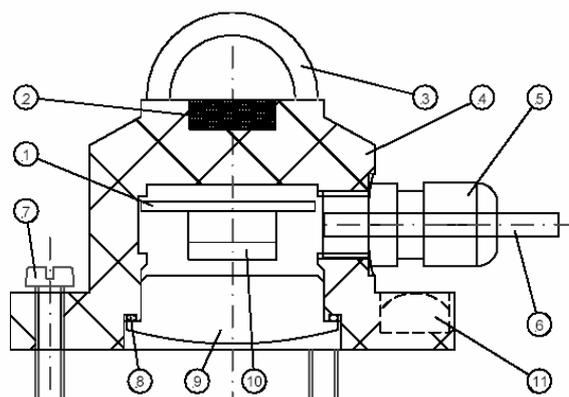
Fig. 2. Working principle scheme of a pyranometer
