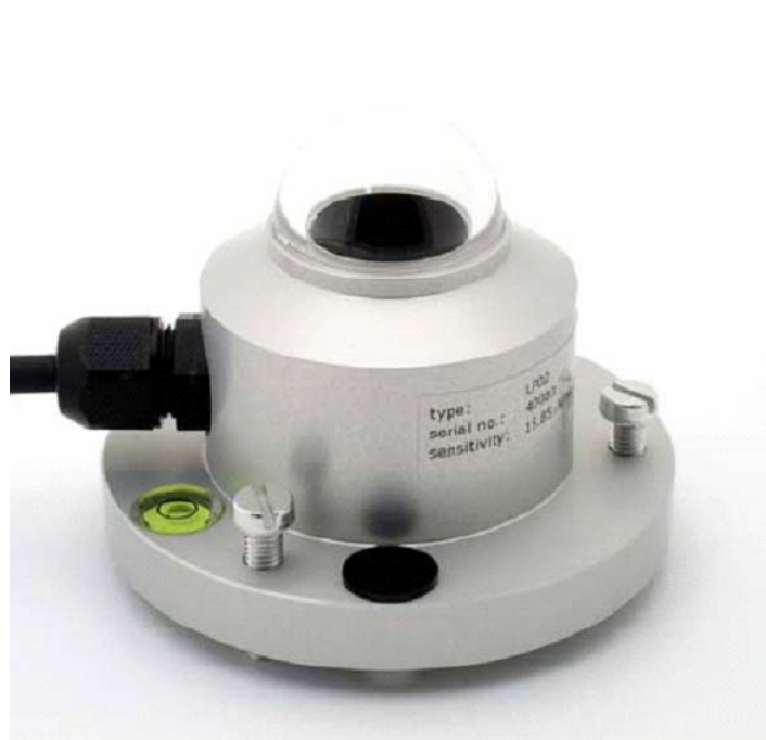
Sensor for solar radiation measurement (pyranometer)
